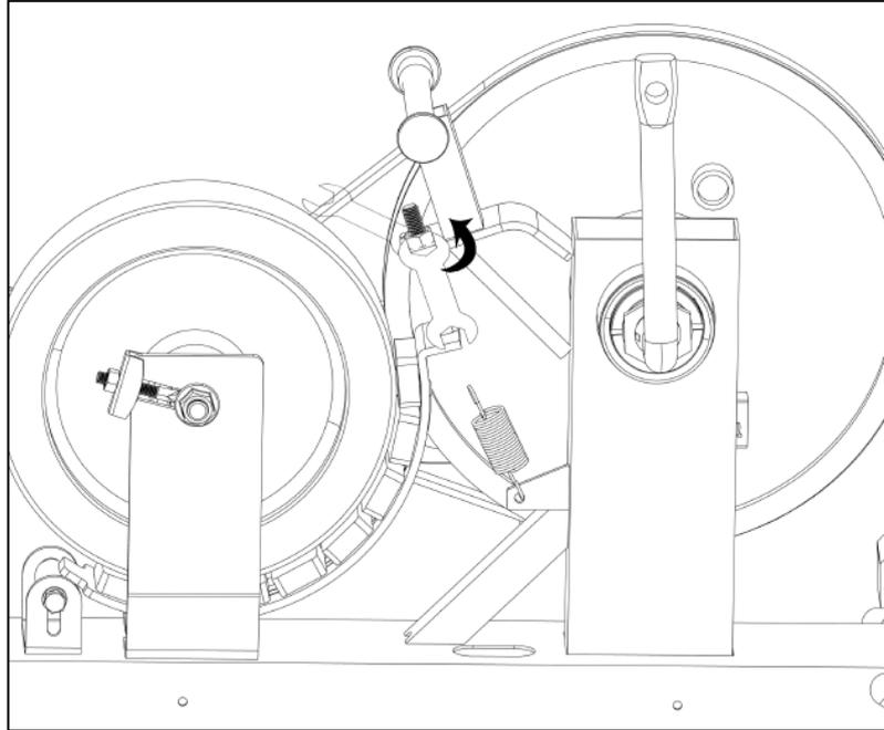
7. If you still hear noises after you did Step 5 and Step 6, please remove the **Belt Cover (No. 65L/R)**. Loosen the screws for the **Flywheel (No. 94)** about a half of a rotation. See the following diagram below.
