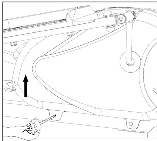
6. If it is very hard to pedal on the higher tension levels, or you hear rubbing noises, please remove the **Belt Cover (No. 65L/R)**, and adjust the screw seen in the following diagram. You will need to lower the position of the screw by turning counter-clockwise. This will keep the **Magnet Board (No. 84)** from contacting the magnetic flywheel. Before re-installing the **Belt Cover (No. 65L/R)**, test the tension level 8 to ensure the magnets do not touch the flywheel.
