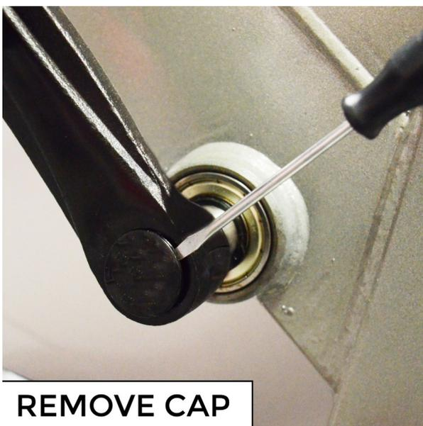
**STEP 2:** Begin the crank removal processes by removing the crank's "cap" piece. You can do this with a flat head screwdriver. This should just "pop" right off.
